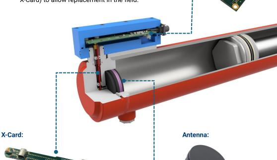
The X-Card is the connection between the external electronics and the internal antenna. Its length varies with cylinder diameter.
